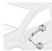
Step 4: We recommend using our body reamer to drill mounting holes.
