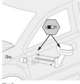
Step 5: Insert the LED connecting wire and fix the wing mirror with screw on the holes which we drilled in Step 4.
