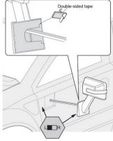
Step 5: Insert the LED connecting wire on the holes which we drilled in Step 4, and fix the wing mirror with double-sided tape.
