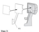
Put the mirror plate on the wing mirror, then stick the silver mirror decal on the mirror plate.
