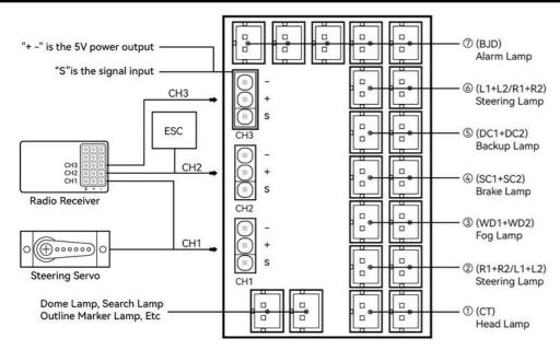
CH1 Channel: Steering Channel (Turn ILeft, Turn Right).
