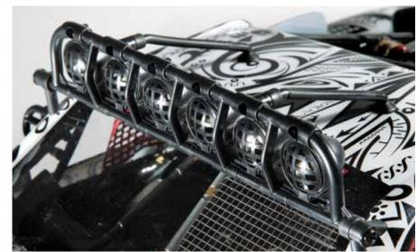
I really like adding lights to scale vehicles and Killerbody has a nice package that will make this short course body stand out from the rest. Light buckets with LED lights are installed to the inside of the body at the rear of the roof line and at the rear of the body. There is also the option of adding the roof light bar that really delivers the message that this short course is now destined for some desert running
