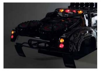
By adding the Killerbody accessories, this short course body is transformed into a very scale looking vehicle. On the rear is the molded spare tire kit that comes clear and includes stickers. The functioning metal ratchet tie-downs help complete the look, but they are not necessary to keep the spare tires in place. Also in this photo is the rear 'X'-shaped roll cage with two fire extinguishers mounted.
